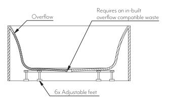
(3)Plan out drainage connection to floor waste & alter if necessary. Fit plug waste (must have overflow) into bath outlet, seat and tighten as required.
