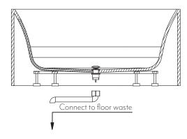
Fit out drainage connection to underside of bath. (4)Position bath & connect drainage to floor waste.
