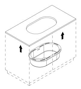
Depending on material of benchtop mount brackets 4 using either 1. adhesive, or 2. provided screws.
