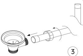
Add rubber seal into the overflow fitting, line up with hole and place on outside of sink. Tighten screw to fix parts together.
