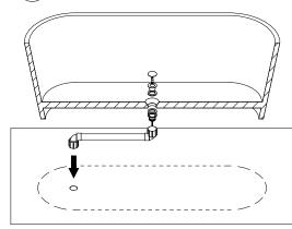
Fit plug waste into bath outlet, seal & tighten as required.
