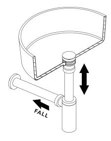
Engage kee seal into 40mm socket.
