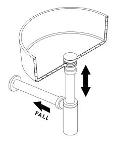
Engage kee seal into 40mm socket.
