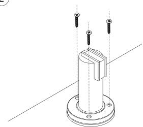
Mark out desired position for door catch in relation to door stop magnet on floor. Drill pilot holes into door.
