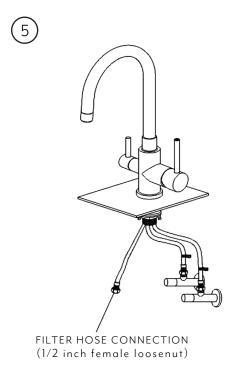
Connect cold line associated with filter handle to filter hose connection
