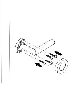
**Note:** If screwing into a hollow core door, screw into solid section to ensure secure installation.
