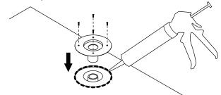
Adjust the top of the puddle flange to the finished height required for the shower grate installation.
