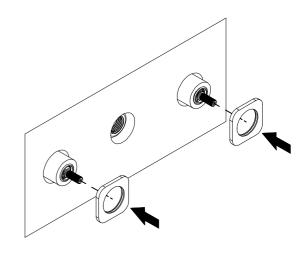
Install handle onto spindle by tightening grub screw with provided Allen key. Insert grub screw cap.
