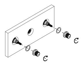
**New build:** Install breech in desired position and arrangement (**Note:** breech sold separately). See following page for setback guides.
