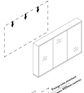
If correct height and position is suitable, level the top of the mirror cabinet & mark out desired position. Drill holes through the back of mirror cabinet into structure within wall using a wood drill bit.
