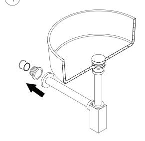
Assemble trap and tighten all components.
