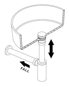
Engage kee seal into 40mm socket.
