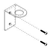
IMPORTANT - If installing onto plasterboard please use appropriate fixings.
