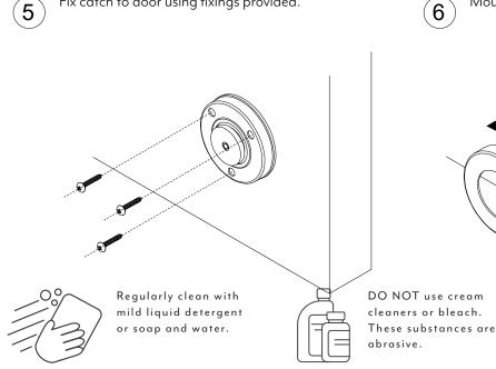
Fix catch to door using fixings provided.
