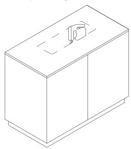
2 Lay a piece of timber across the benchtop hole & position in line with trough hole below.
