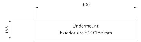
UNDERMOUNT INSERT TEMPLATE- refer to install method 3
