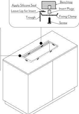
Undermount Fixing Detail
