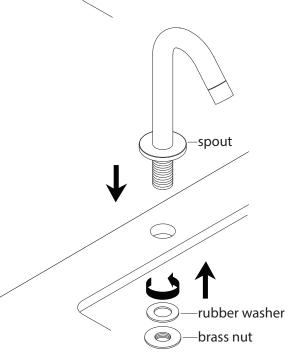
Fix spout to benchtop with brass nut ensuring rubber washer is fitted to underside of benchtop.
