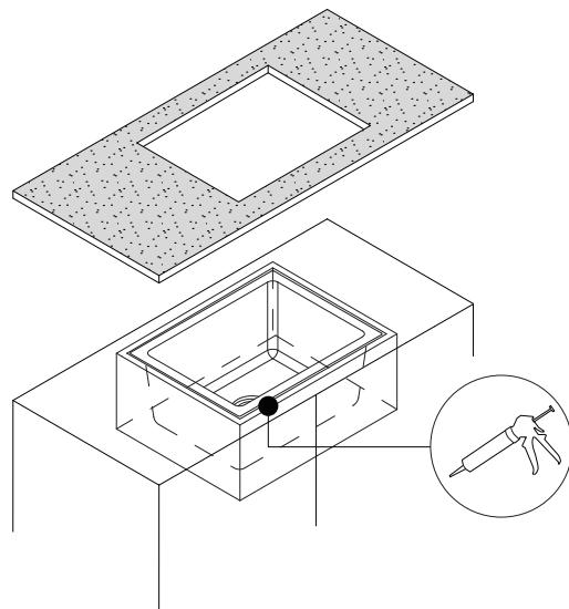
**4** Install the benchtop & apply adhesive to sink perimeter. Wipe away any excess adhesive sealant.
