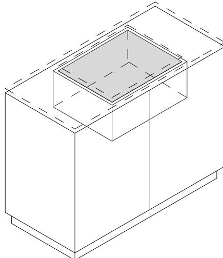
**2** Mount the sink into the cabinet box. **Ensure the top of the sink is flush with the top of cabinetry.**
