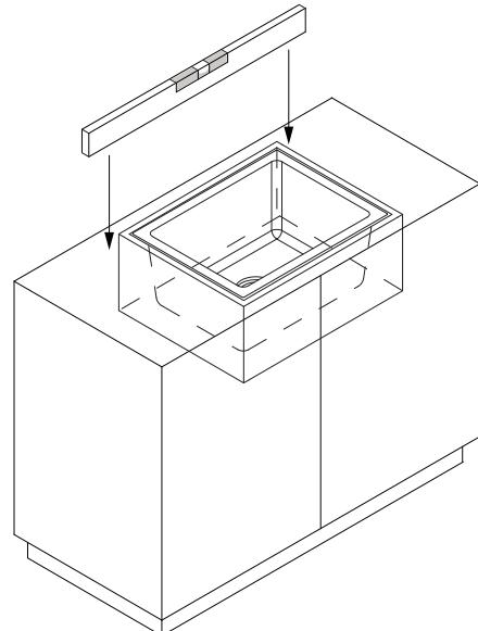
**3** Cut the benchtop using the internal measurements of the sink perimeter in conjunction with the desired sink overhang.
