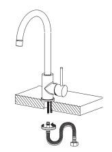
Place the mixer connections through the hole in bench. Pass the horseshoe plates over the bolts on the underside of bench, fasten the nuts and tighten.
