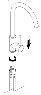
4 Connect the two flexible hoses into the water supply by hand tightening & making a final adjustment with a spanner.
