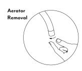
**Note:** WELS star rating does not apply when non-restricting aerator is installed.
