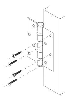
Fix the hinge to the door jamb using fixings provided.
