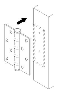
Align the hinge with the door jamb and mark out fixing locations.
