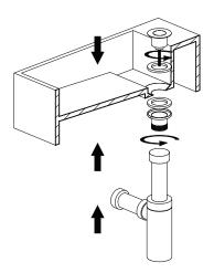
Hold basin against wall aligning outlet of trap with waste pipe. Extend telescopic trap up or down to find desired height & cut waste to suit trap.
