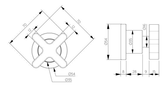
Note: Spindle & spindle body (in wall) not included in handle kit
