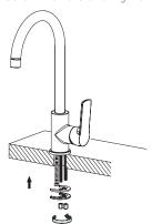
Attach the two flexible hoses to water supply.
