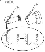
Cut the protective sleeve. Apply lubricant to deburred edges.
