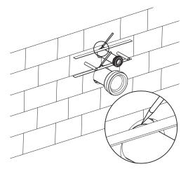
Apply lubricant on rubber washers of straight tube and connecting pipe, then insert into pan.
