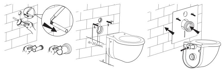
Mount and secure pan according to pan instructions. Apply silicone. Test and commission.
