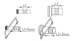
Deburr edges of the cut surface of the
