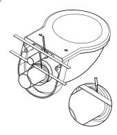
Measure the distance between the 2 marked lines on the straight tube, add 5mm and cut. Measure the distance between the 2 marked lines on the straight tube, add 3mm and cut.
