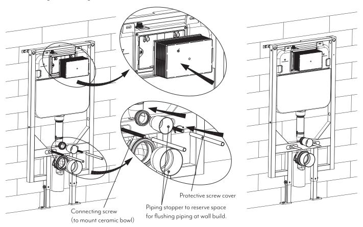
(6) Finish the wall. The finished wall thickness must be between 20-60mm.
